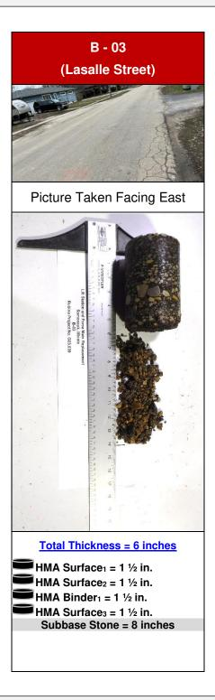
The referenced thicknesses are considered approximate. Commentary provided by Rubino is based on our observation in the laboratory; **Crack** = vertical through cross section; **Weathering** = rounded edges & degradation of asphalt and **Deterioration** = horizontal crack. Pavement and subbase type and thickness may vary between core locations. Any comments on the condition of the material are considered our opinion and should be verified by the design engineer.
